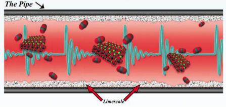
Hydrokon treats fluids by inducing a electrostatic field of 7k to 12k DC volts, yet harmless fields throughout plumbing pipe lines/systems made of any material, including PVC. When the Hydrokon signal is present, dissolved minerals combine to form loosely held clusters.
